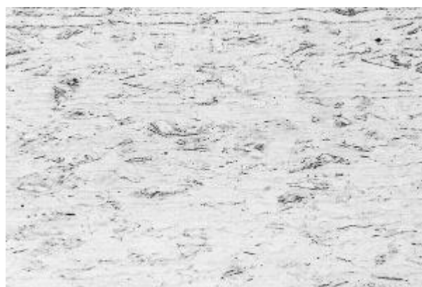
FIGURE 20 | Structure with carbide precipitation
