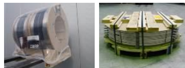
FIGURE 11 | Special packaging: Coils and multicoil, inner and outer packaging and crate
