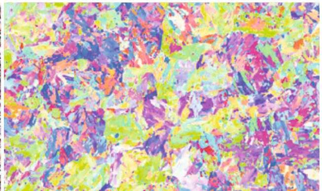
Crystal orientation map of hardened and tempered Zapp 1.4028MO
